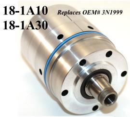
The motor is of the orifice bearing type that allows the shaft/flywheel/bell cup assembly to "float" frictionless on a thin film of air. Drive air (DA), brake air (BR), turbine exhaust (EX) as well as the bearing air (BE) are supplied to the motor assembly via the back plate.
