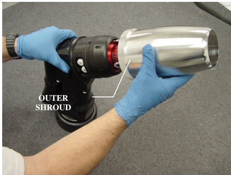
Figure 18: OUTER SHROUD REMOVAL
