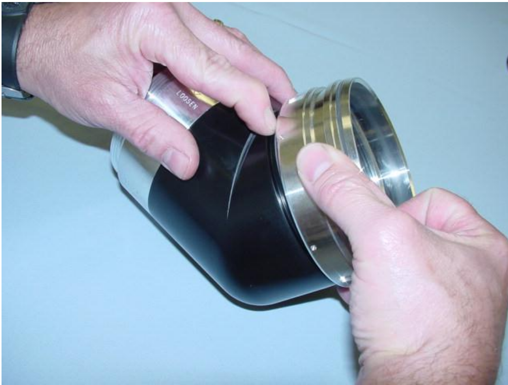
Figure 14: Q. D. Nut Installation
