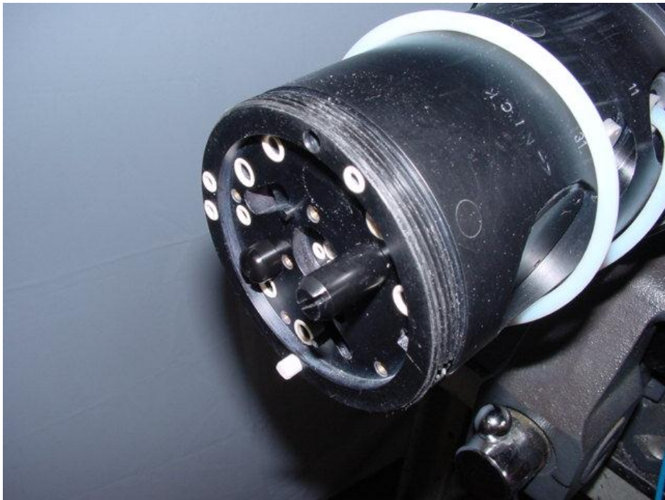
Figure 22: FS67 Installation Onto A Sames 607 Manifold
