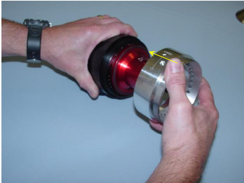
Figure 12: Motor Nut Installation
