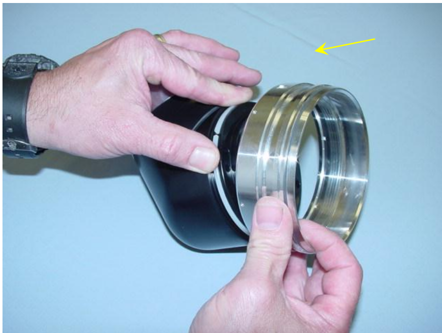
Figure 13: Split Ring Installation
