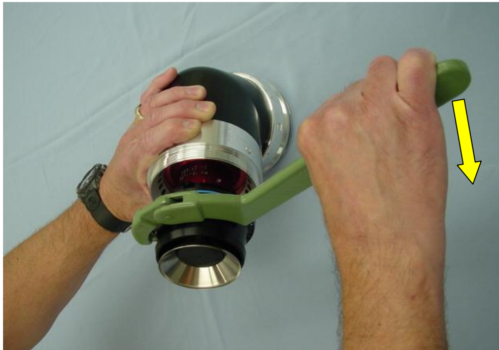
Figure 17: Inner Shroud Installation
