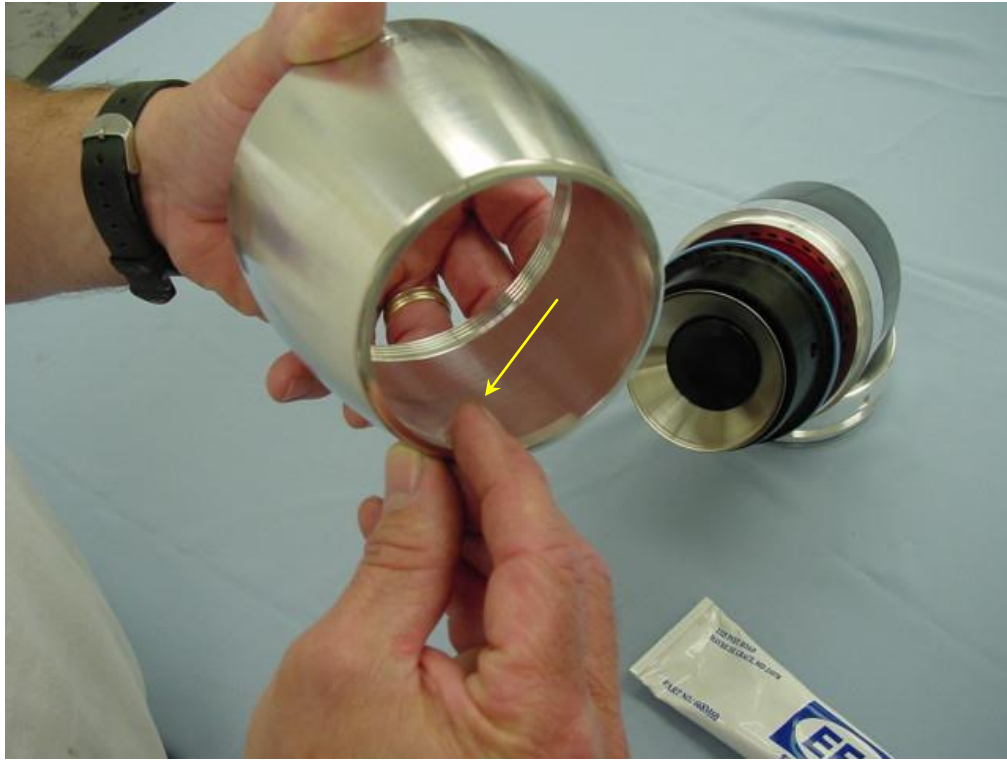
Figure 18: Outer Shroud Installation
