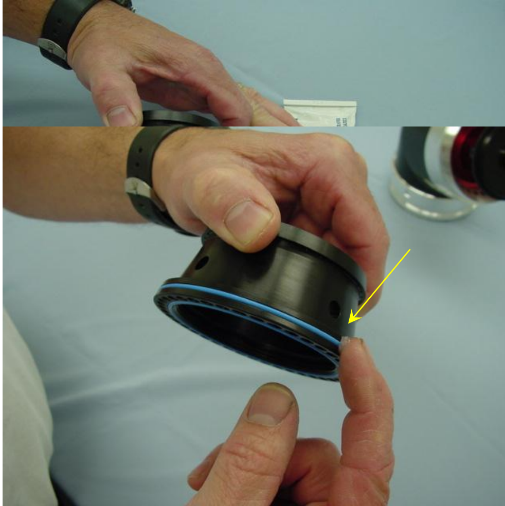
Figure 16: Inner Shroud Lubrication
