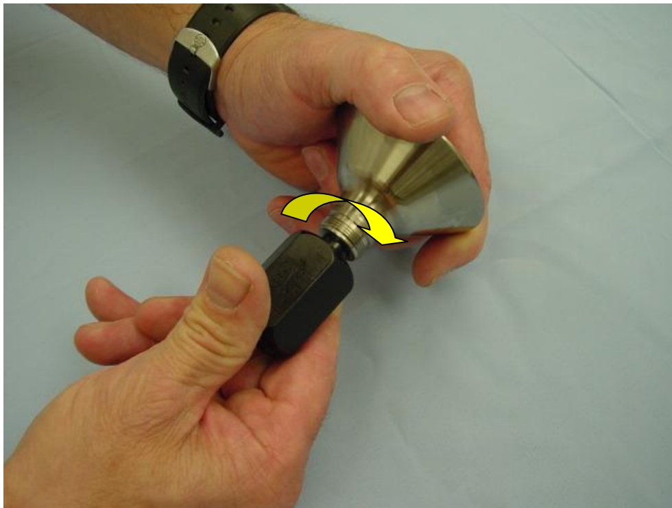
Figure 23: Bell Cup Insert Removal
