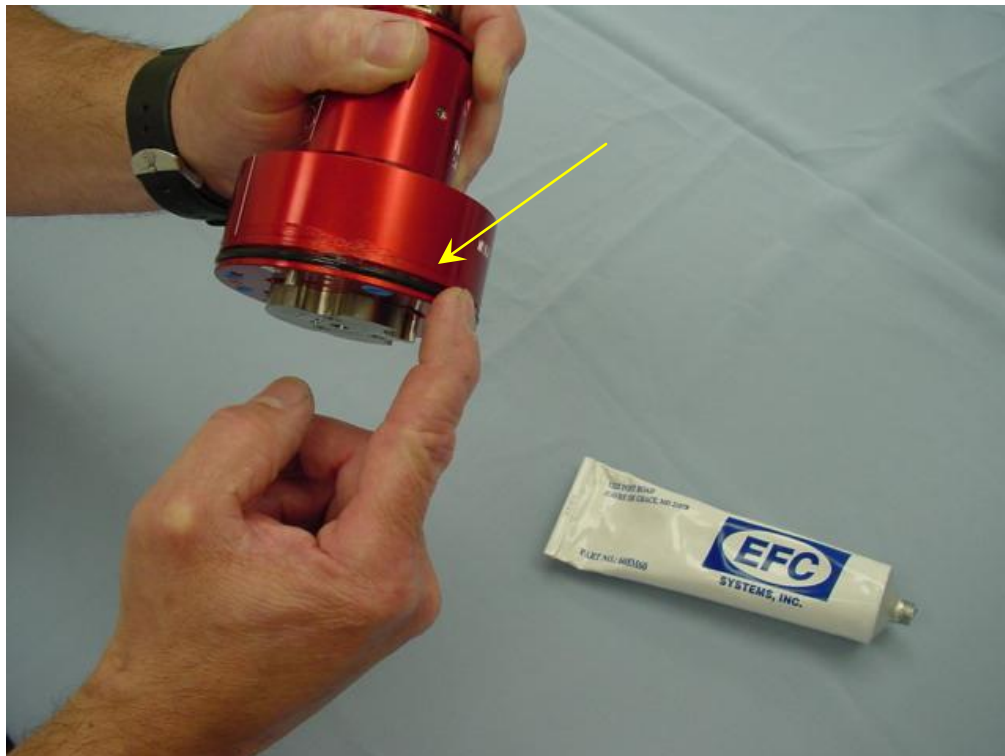
Figure 10: Vaseline® on Motor O-Ring
